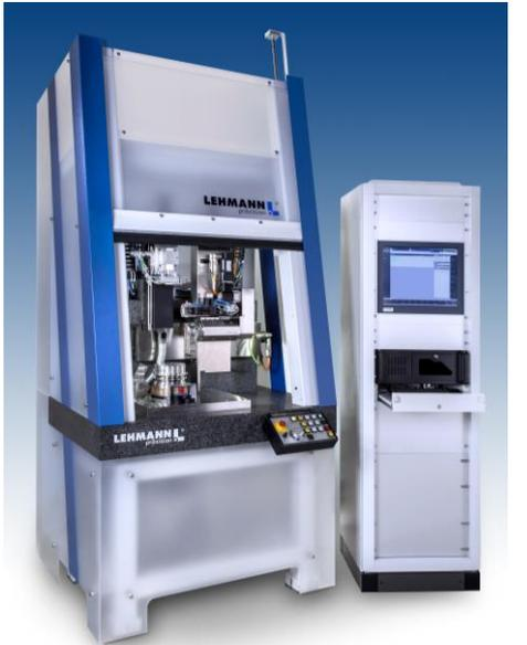
Vertical lathe for lens production
