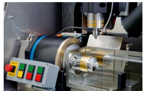
CNC milling machine for gold working
