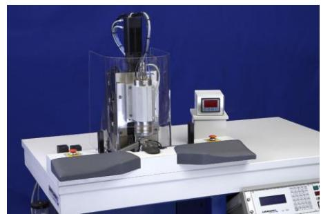
CNC precision milling machine for microparts
