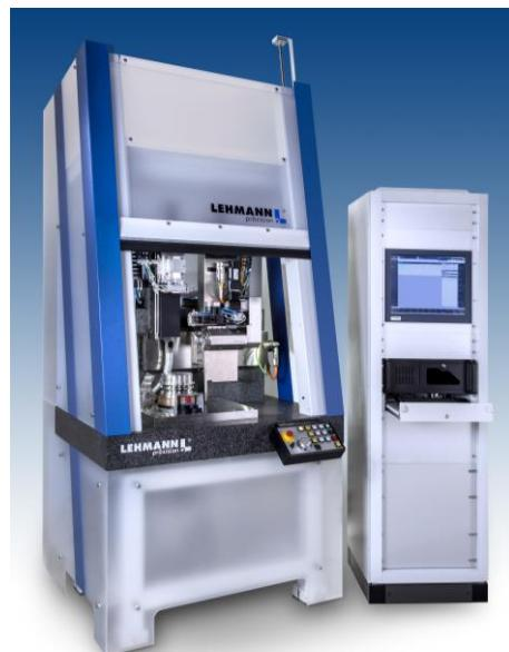
Vertical lathe for lens production
