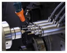
Our spindle program is rounded off by spindles with air bearing reaching speeds of even up to 96,000 min<sup>-1</sup>.
