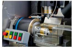
CNC milling machine for gold working
