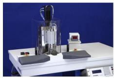
CNC precision milling machine for microparts
